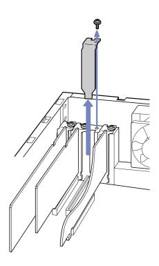
Install the add-on board by plugging it into the expansion slot and secure it with the screw from the expansion slot, as shown:
